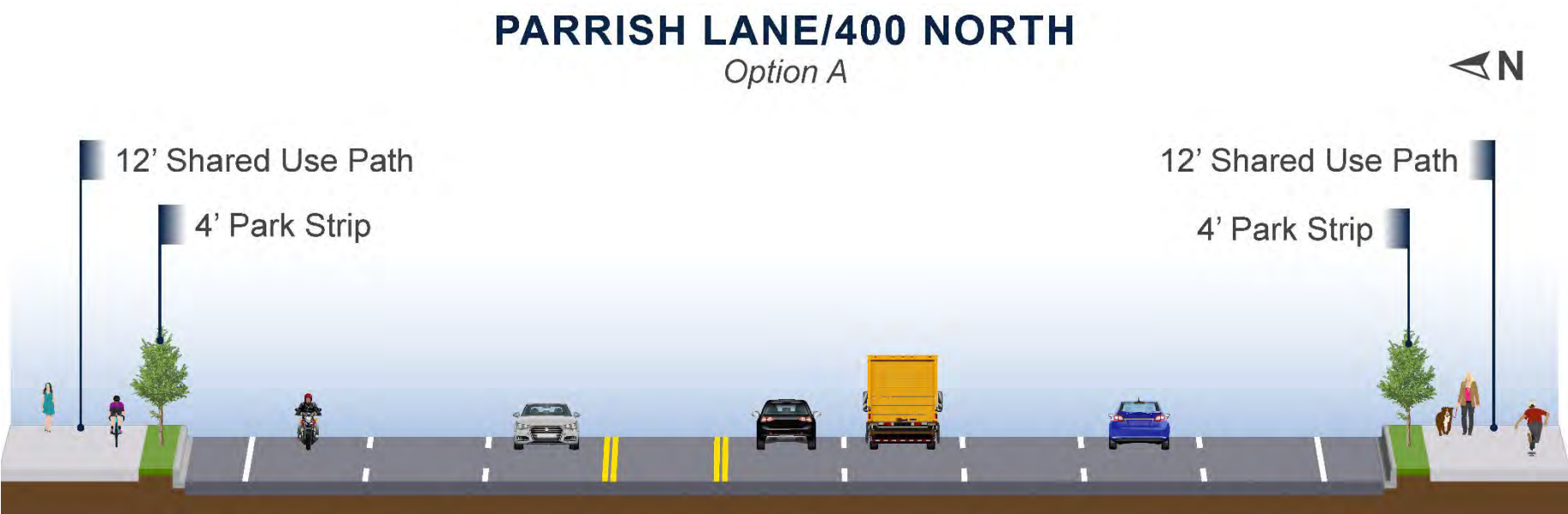
Figure A-29. Cross Section for Parrish Lane/400 North Option A Centerville
