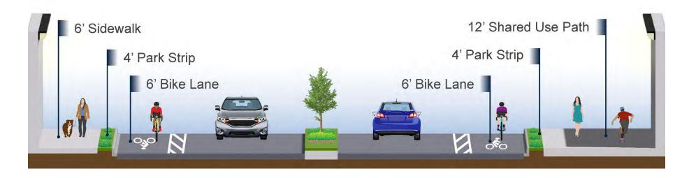
Figure A-14. Cross Section for Main Street in North Salt Lake (for North Salt Lake/Woods Cross Options A and B)
