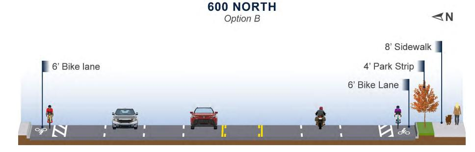
Figure A-7. Cross Section for 600 North Salt Lake City Option B Shared-use Path
