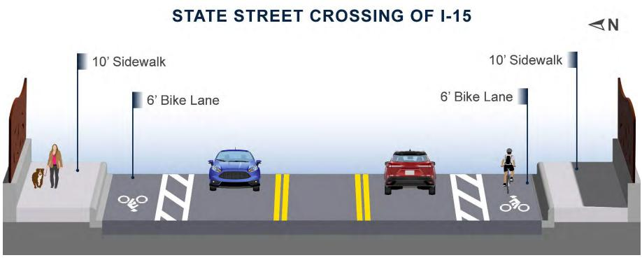
Figure A-36. Cross Section for Shared Use Path Farmington Option B
