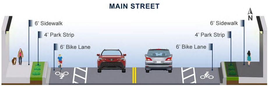
Figure A-15. Cross Section for North Salt Lake/Woods Cross Option A
