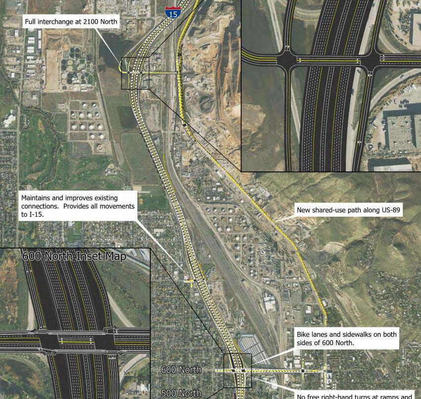
Figure A-40. Salt Lake City Option A 600 North CD and 2100 North Full Diamond Interchange (Reversible I-15 Mainline)
