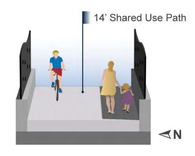
Figure A-31. Cross Section for Porter Lane Pedestrian and Bicyclist Crossing Centerville Option A
