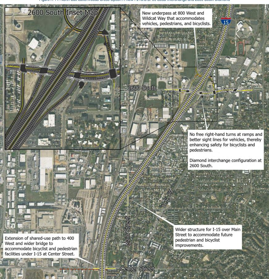
Figure A-11. North Salt Lake/Woods Cross Option A New I-215/U.S. 89 Local Interchange and 2600 South Diamond
