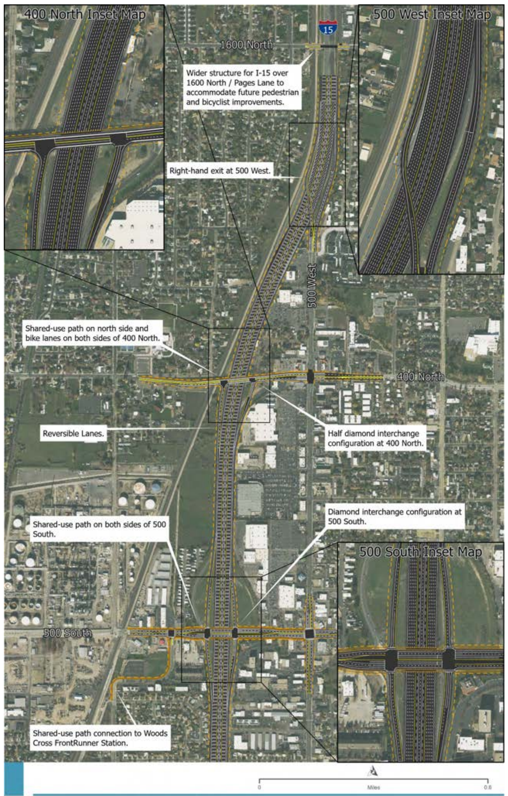
Figure A-44. Bountiful/West Bountiful Option A 500 South Diamond and 400 North/500 West Half Diamond (Reversible I-15 Mainline)
