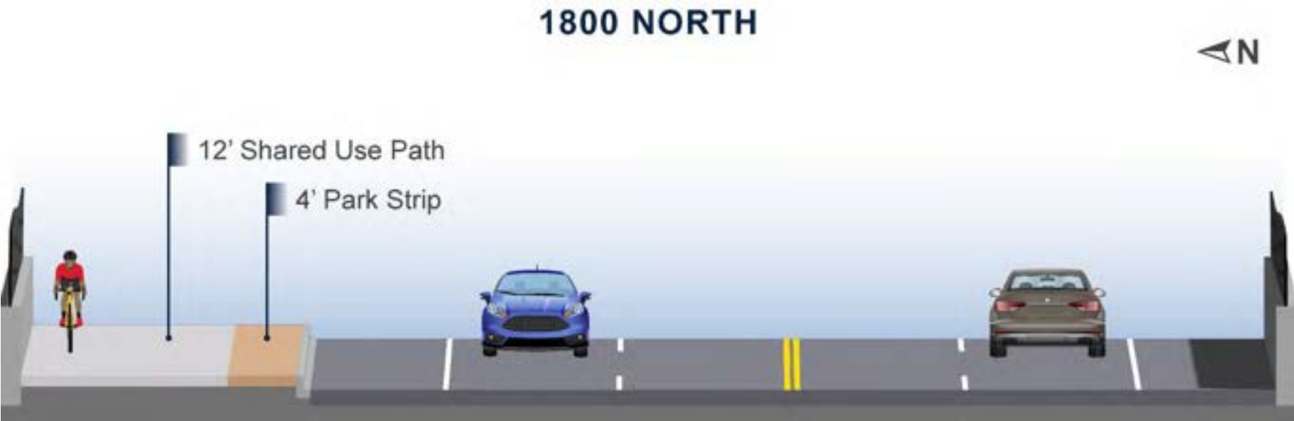
Figure A-10. Cross Section for 1800 North Bridge for Salt Lake City Option B
