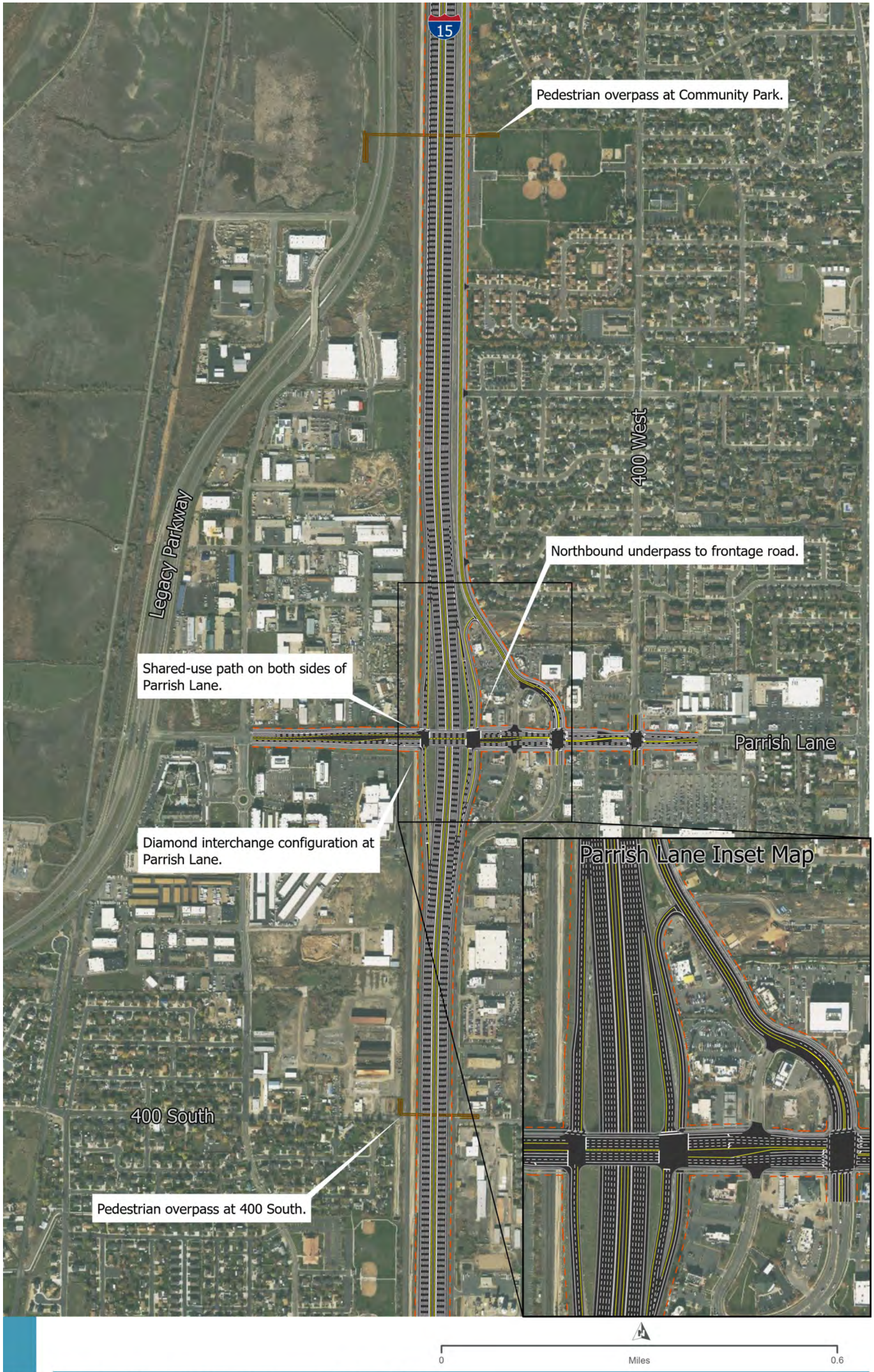
Figure A-27. Centerville Option A Parrish Lane Diamond with NB Connection to East Frontage Road
