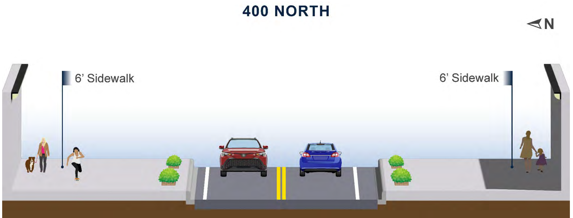
Figure A-4. Cross Section for 400 North Salt Lake City Options A and B
