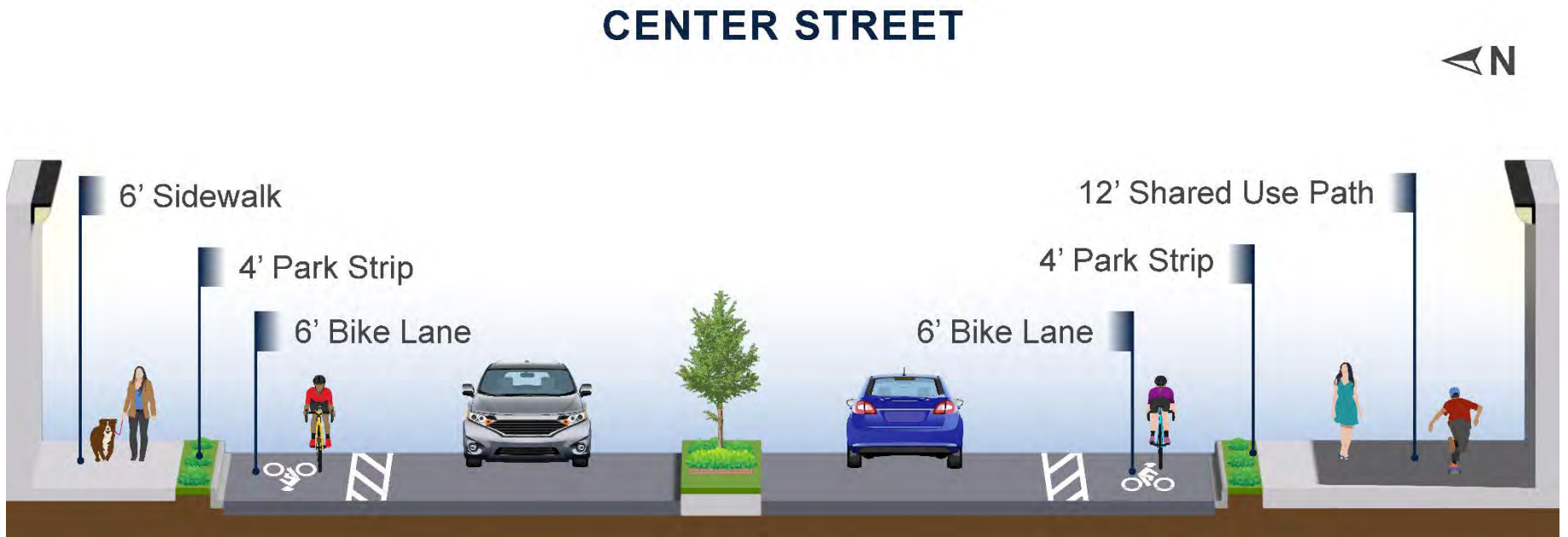
Figure A-13. Cross Section for Center Street in North Salt Lake (for North Salt Lake/Woods Cross Options A and B)
