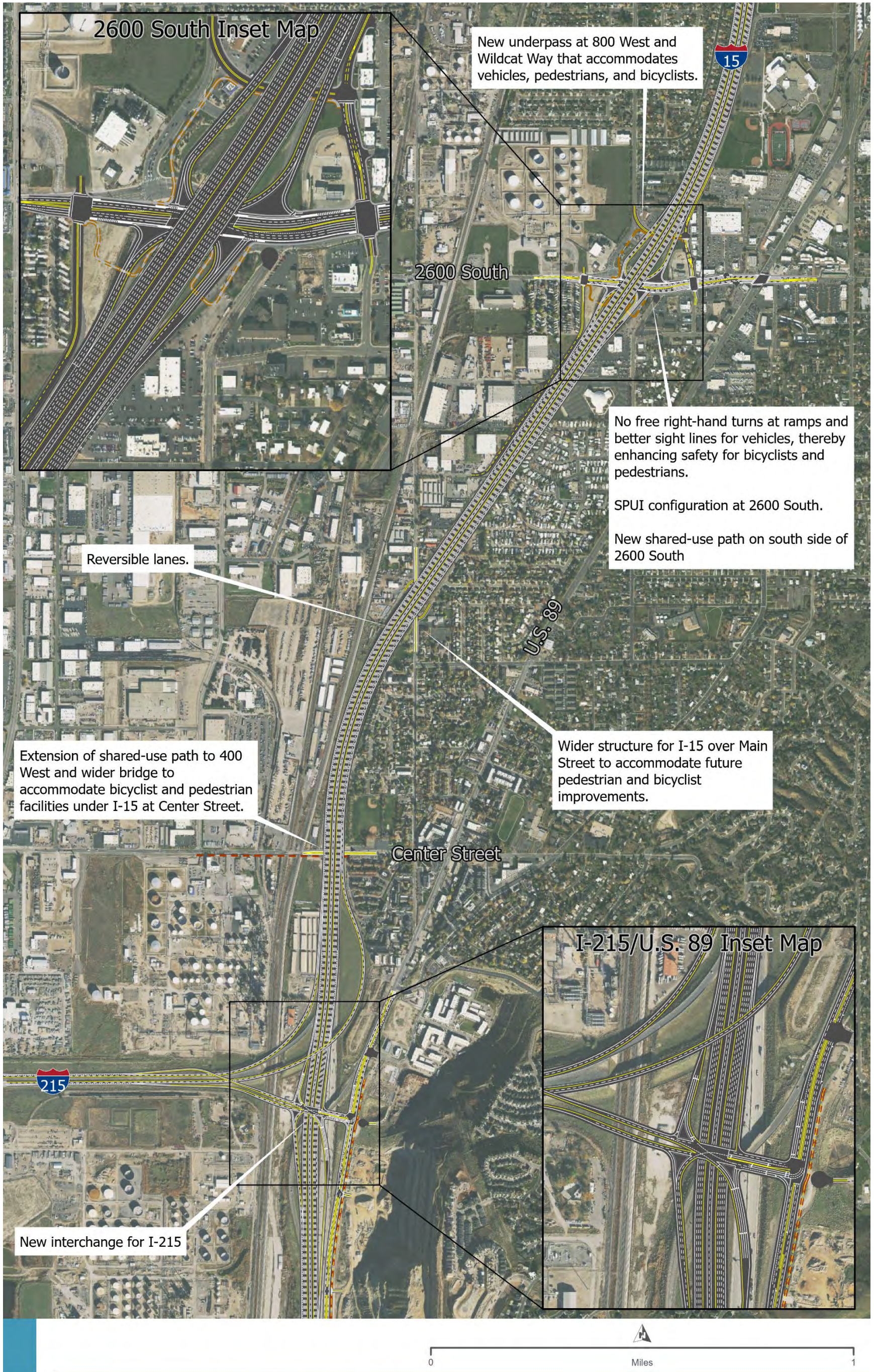
Figure A-43. North Salt Lake/Woods Cross Option B New I-215/U.S. 89 Local Interchange and 2600 South SPUI (Reversible I-15 Mainline)
