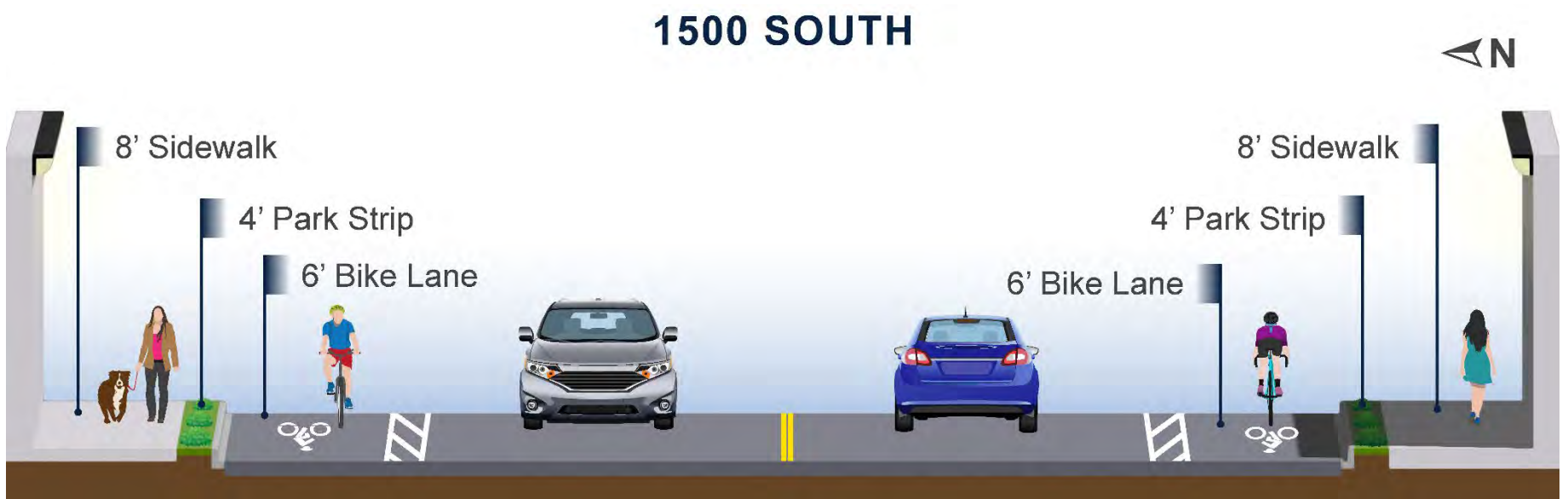
Figure A-19. Cross Section for 1500 South Woods Cross (for North Salt Lake/Woods Cross Options A and B)
