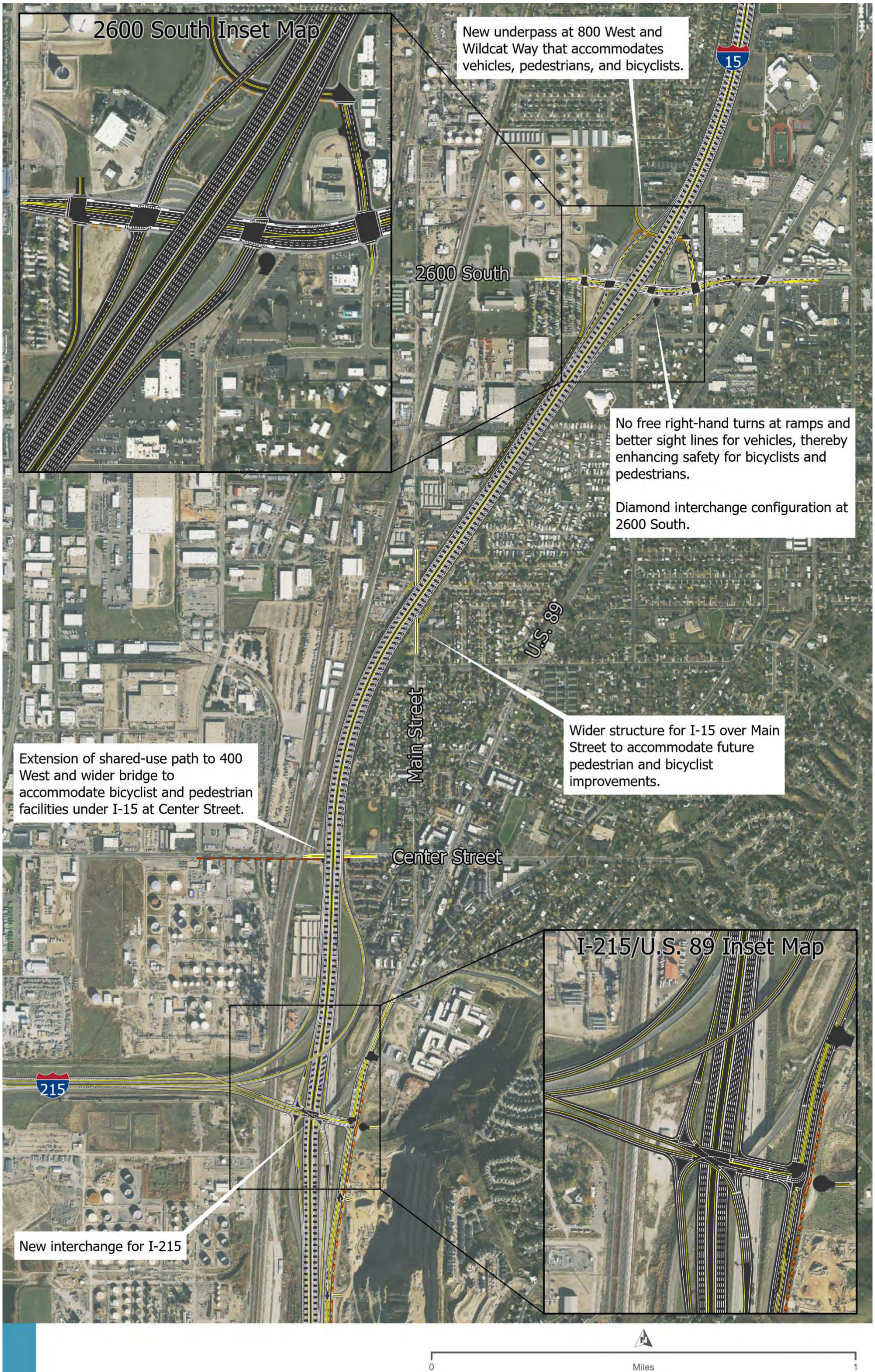
Figure A-11. North Salt Lake/Woods Cross Option A New I-215/U.S. 89 Local Interchange and 2600 South Diamond
