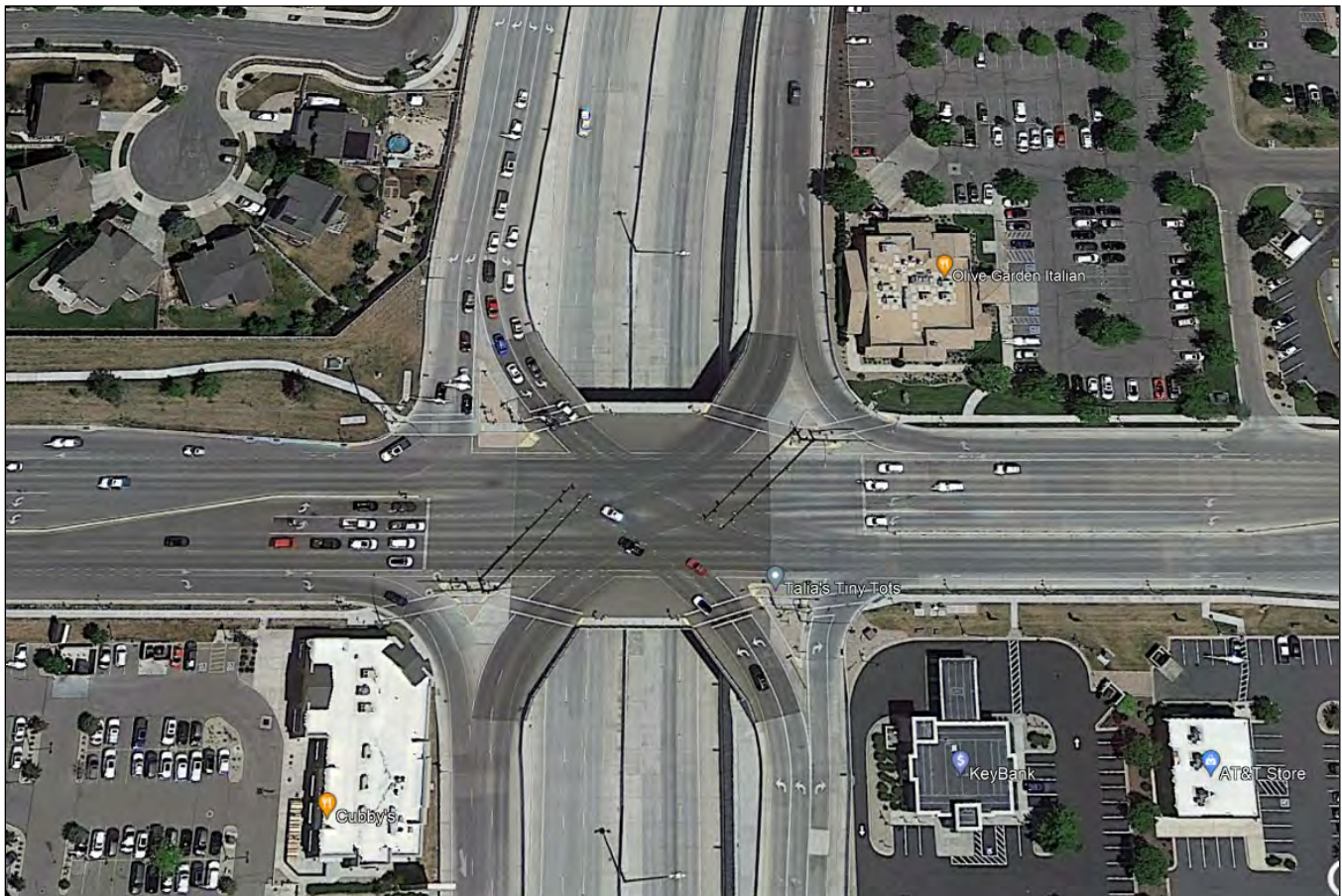
Figure 3-8. Aerial View of SPUI Example on Bangerter Highway and 11400 South in South Jordan
