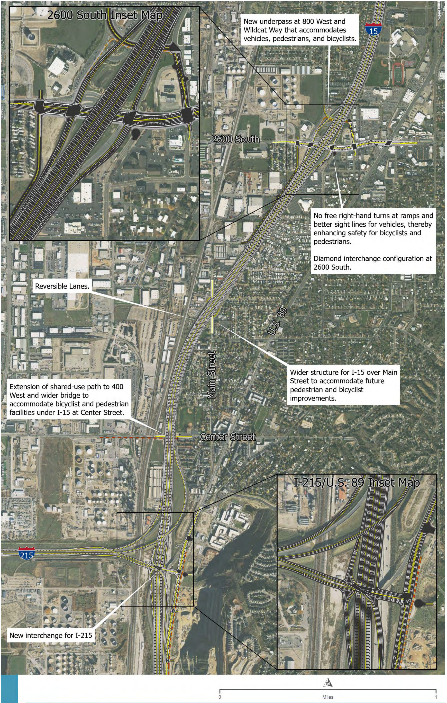
Figure A-42. North Salt Lake/Woods Cross Option A New I-215/U.S. 89 Local Interchange and 2600 South Diamond (Reversible I-15 Mainline)
