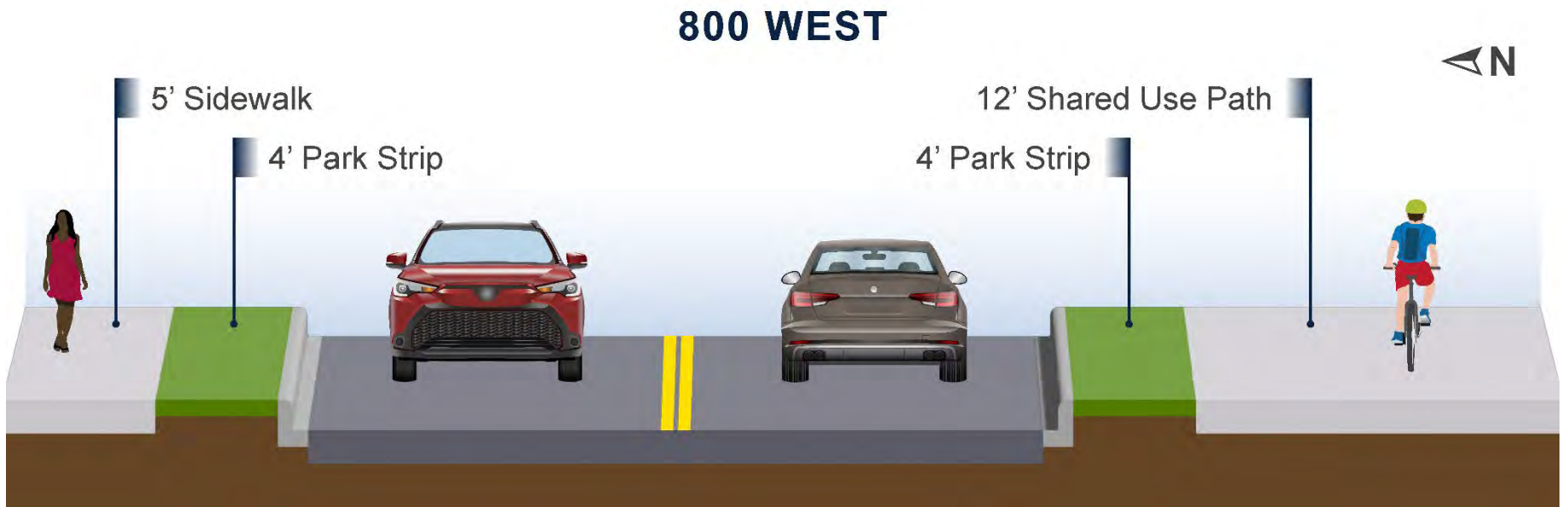
Figure A-18. Cross Section for 800 West for North Salt Lake/Woods Cross Option A and B
