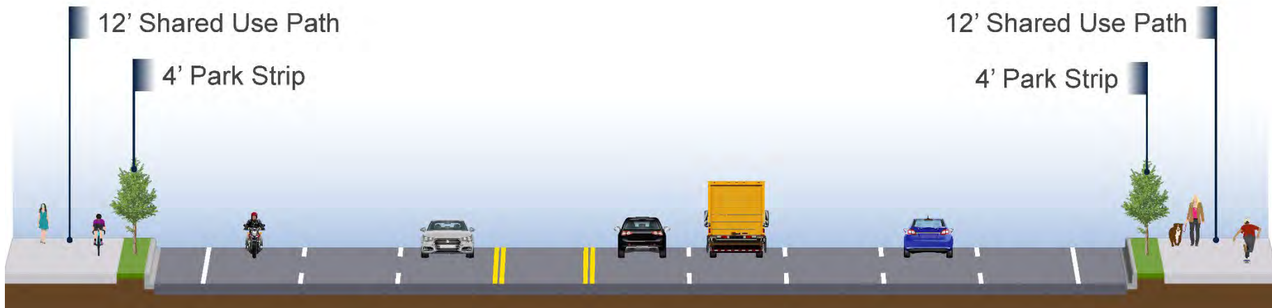
Figure A-30. Shared Use Path Cross Section for Parrish Lane/400 North Option B Centerville
