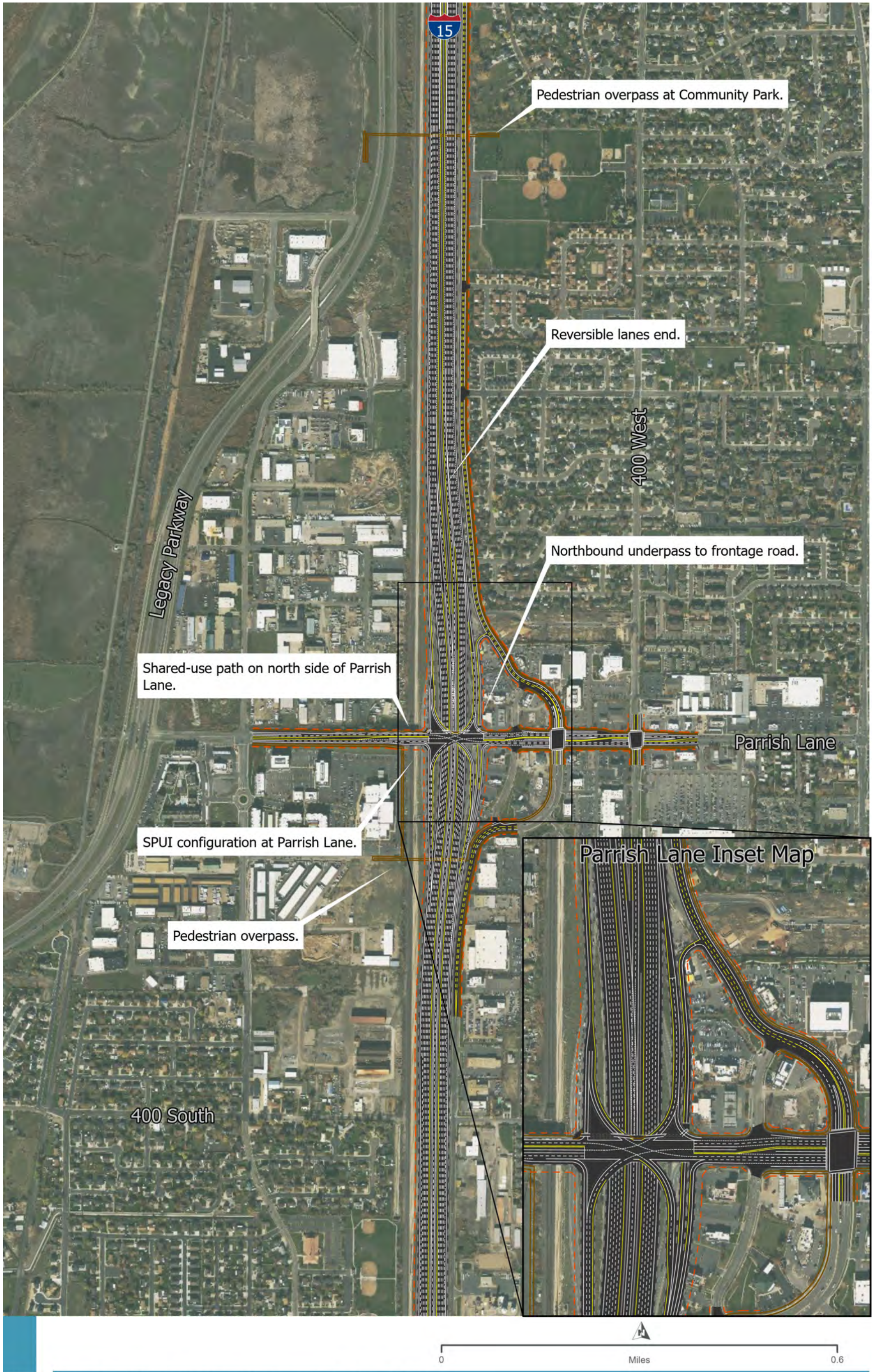
Figure A-48. Centerville Option B Parrish Lane SPUI with NB Connection to East Frontage Road (Reversible I-15 Mainline)
