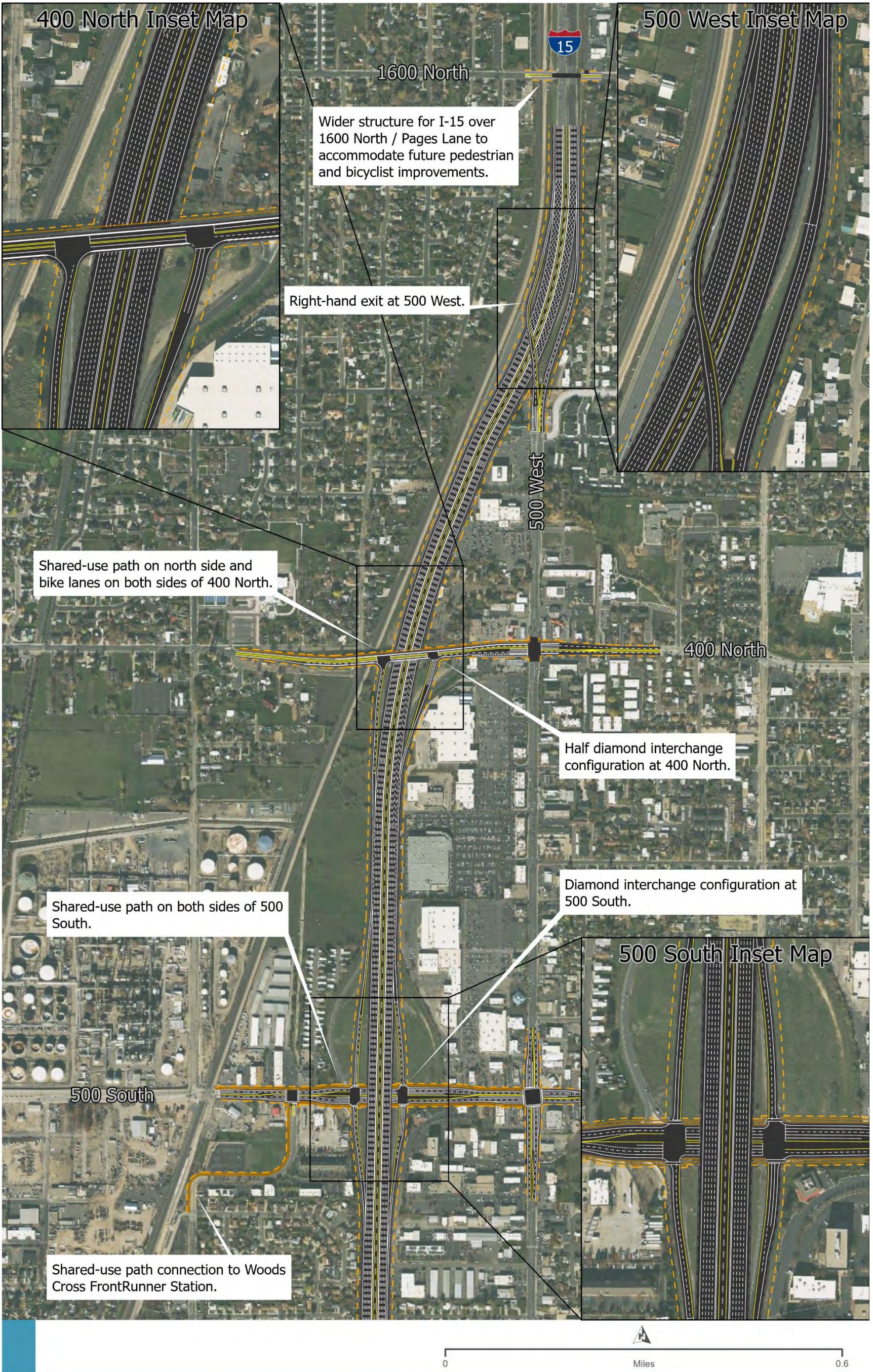
Figure A-20. Bountiful/West Bountiful Option A 500 South Diamond and 400 North/500 West Half Diamond
