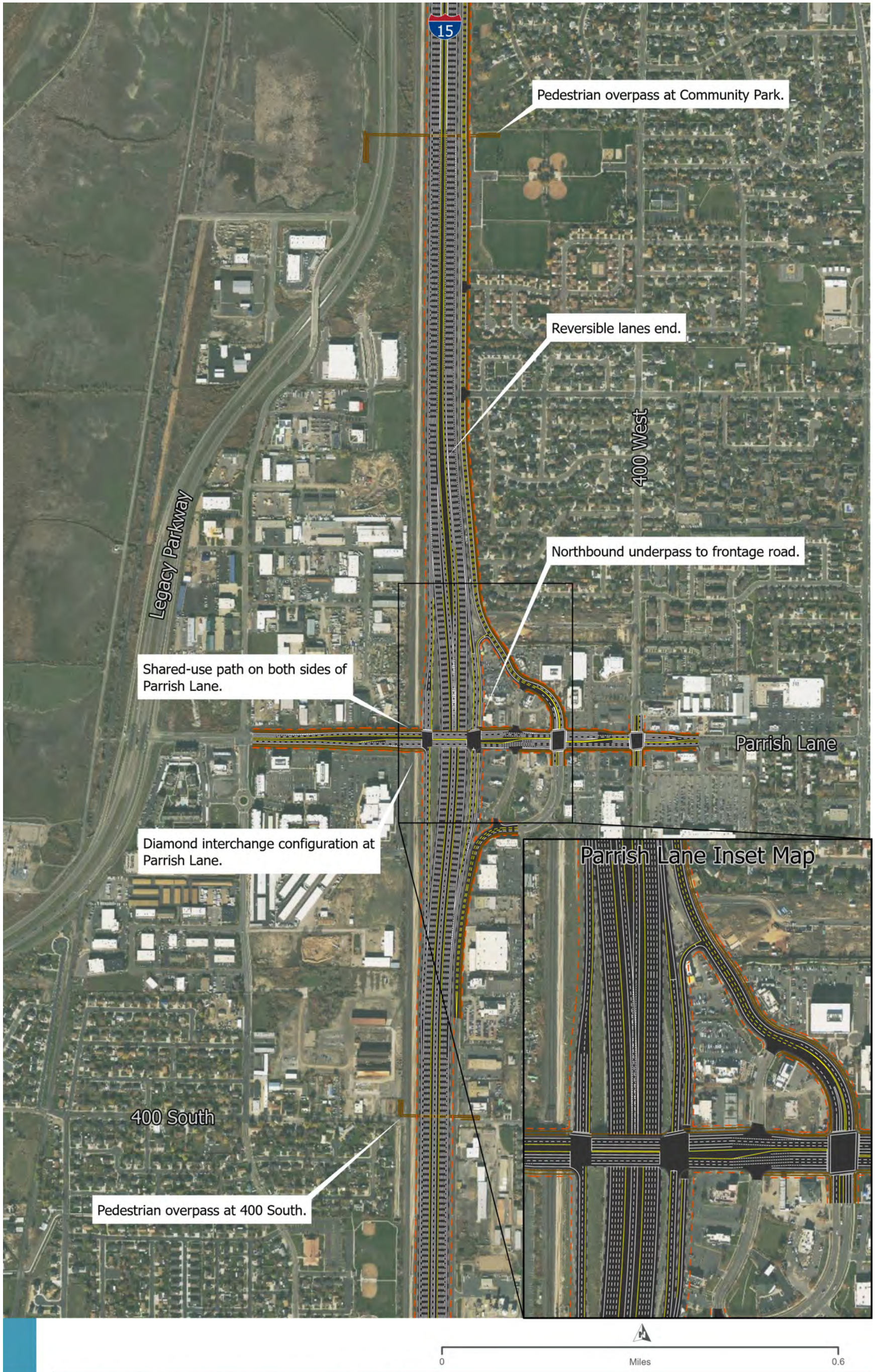
Figure A-47. Centerville Option A Parrish Lane Diamond with NB Connection to East Frontage Road (Reversible I-15 Mainline)
