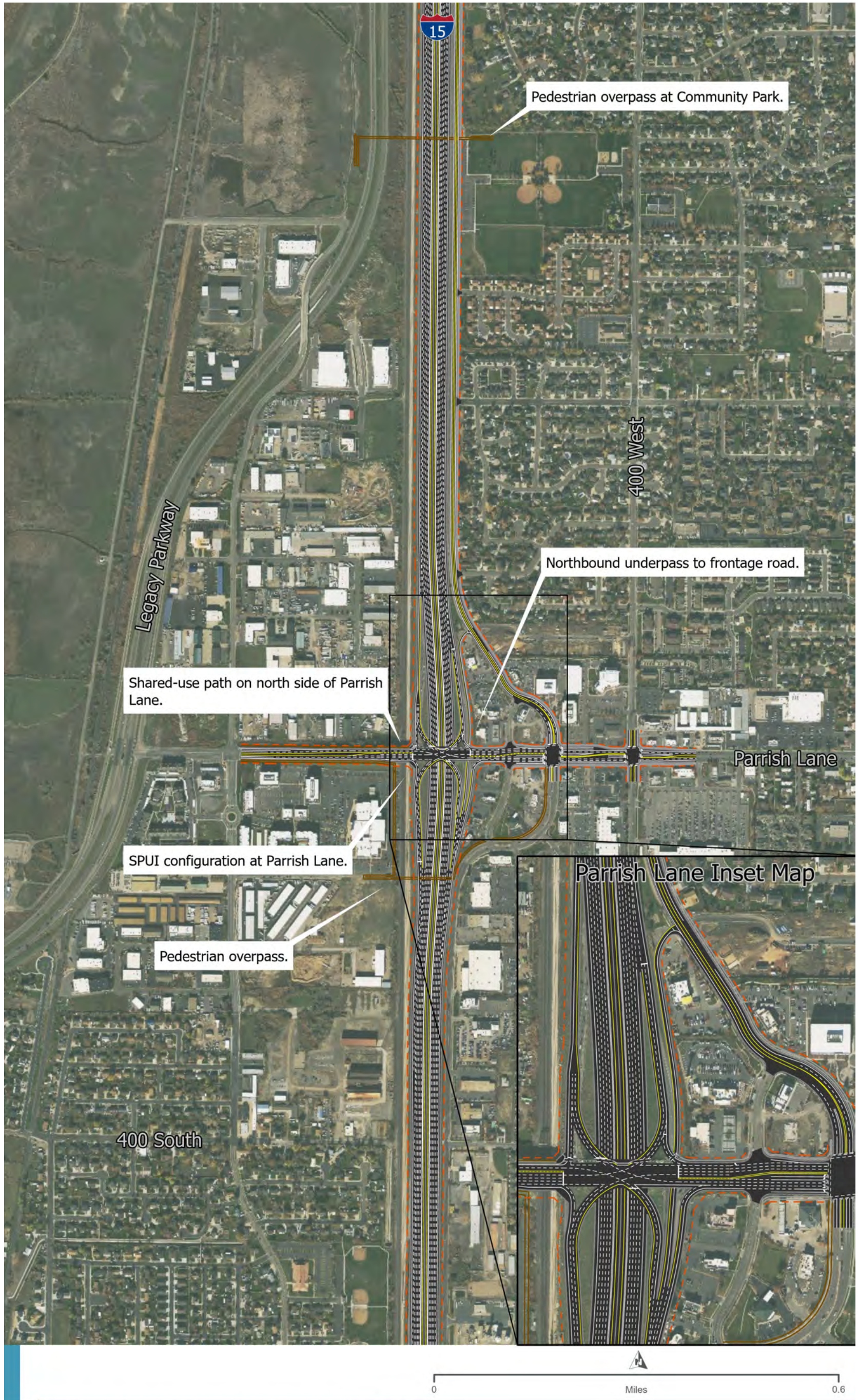
Figure A-28. Centerville Option B Parrish Lane SPUI with NB Connection to East Frontage Road
