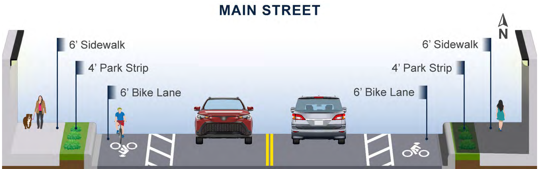
Figure A-14. Cross Section for Main Street in North Salt Lake (for North Salt Lake/Woods Cross Options A and B)
